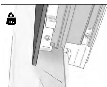
► Gently pull the sash towards you at the top, the sash will lean in approximately 25-30° before engaging on restrictors located at both jambs. Carefully release both restrictors by pushing the restrictor arm upwards. The sash will then be released.
