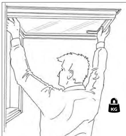
► Open the window to a horizontal position and lift it off.
