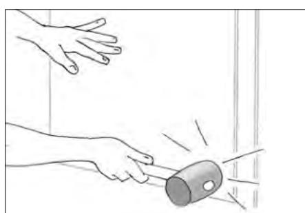
► After ensuring all the clip fittings are in place, knock the backboard in to place using a rubber hammer.
