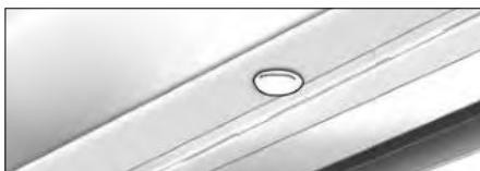
► **Dismounting of the fixed sash.** Locate the long VELFAC Allan key on the glazing of the sliding door or a fixed sash within the delivery. Remove the internal cover cap in the top frame and loosen the 3mm Allen key fitting by turning it 90°. Now loosen the window hardware located around the sash by firmly locating the Allen key into the head of the allen key fitting and turning 90°.
