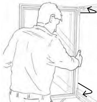
► **Move the sash to the guide rail opening and pull it out.**
