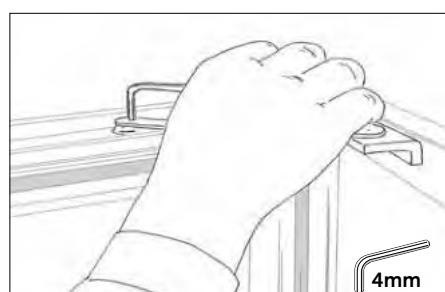
► **Adjusting the friction arm:** Loosen or tighten the screw at the top and bottom of the window sash.
