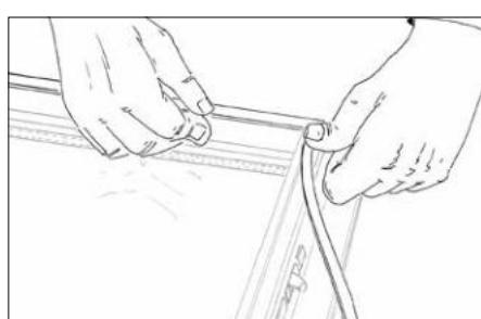
► Press the glass gasket in, starting at the corners, and then proceeding on the sides. Be careful not to twist the gasket.
