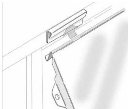
► Push the panel up beneath the fitting. Adjust sideways.
