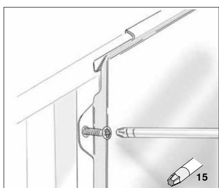
► Press the panel against the frame and tighten the screws at a sloping angle.
