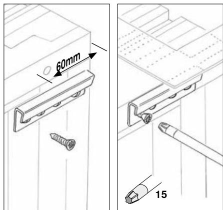
► **Installation of separate panels:** Screw in the fitting at the top, ensuring that it will flush with the edge of the head.
